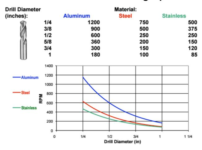
All holes 1/2" or greater should be drilled in 1/8" increments, starting with 3/8"
